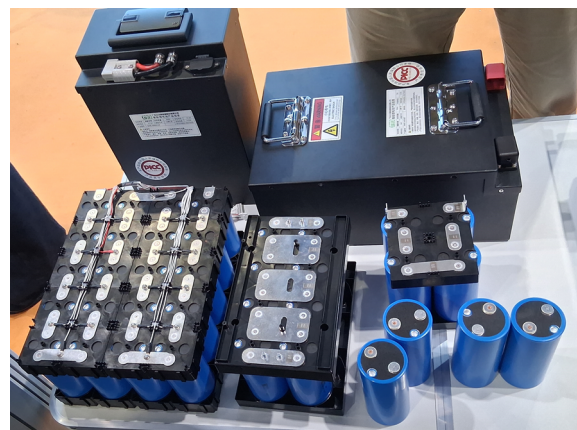
BIWO's high capacity 60140 cylindrical cell. 6
